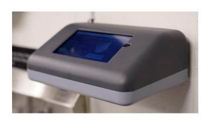
The PathSpot hand scanner is a patented data collection tool that provides instant feedback on handwashing frequency and effectiveness. The hardware unit and proprietary software leverage visible light fluorescence spectroscopy to perform detection of gut biome molecules on hands. Data is displayed both on the screen of the device and on a cloud-hosted data dashboard to allow goal setting and active monitoring of hand hygiene activities.
